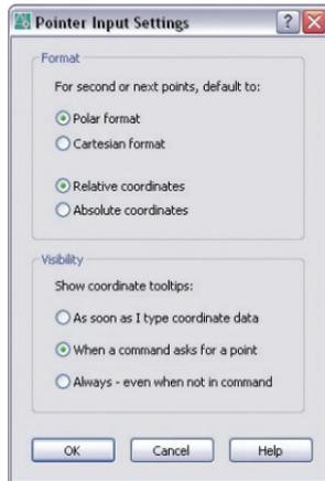
Creating existing geometry and grip editing now allows you to change the length or angle of existing objects by directly inputting the new value on the screen. "Enable dimension input where possible" needs to be toggled on for this to occur. Note: Use the tab key to toggle between the two values.
